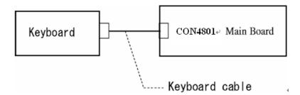
If the connection is loose, reconnect firmly. If there is still an error, go to Check 2.
